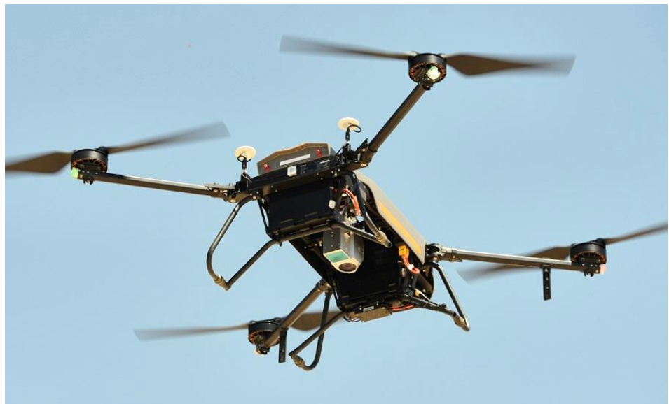
Figure 2. BB4 UAV and AA450 LiDAR scanner performing aerial survey
